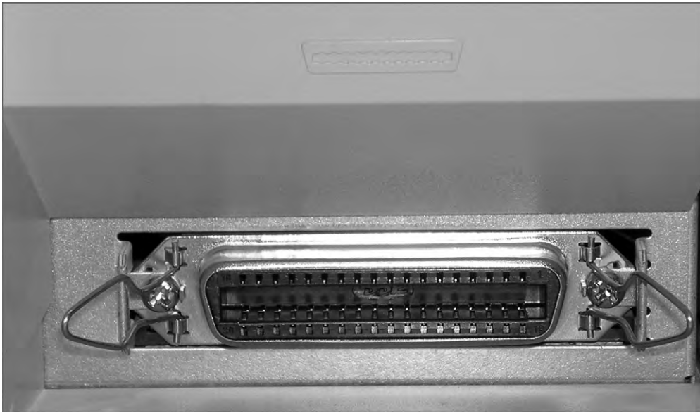
FIGURE 3.15 A Centronics connector
