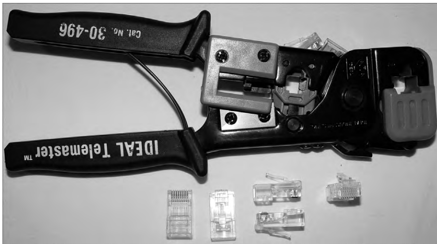
FIGURE 6.24 A UTP crimper
