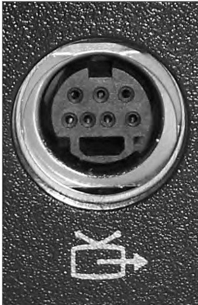
FIGURE 3.40 A 7-pin S-video port
