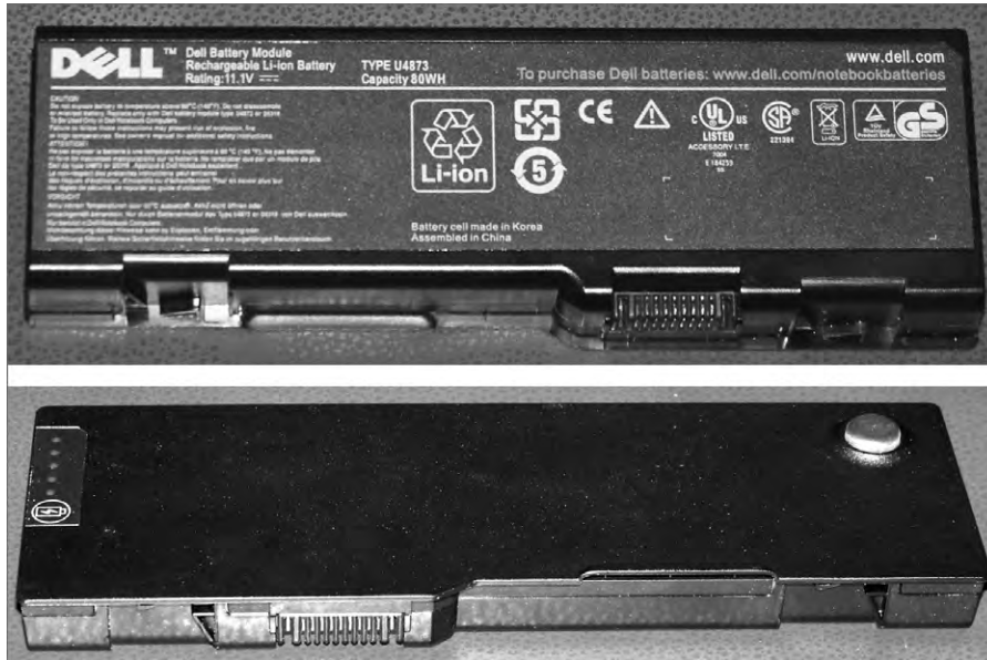
FIGURE 9.17 A laptop Li-ion battery
