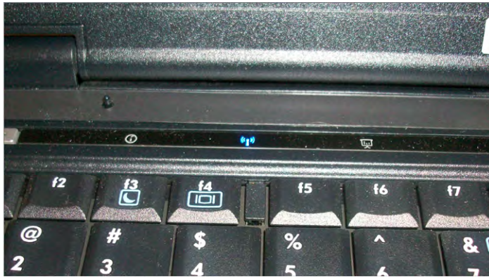
FIGURE 9.12 Network card toggle switch above the keyboard
