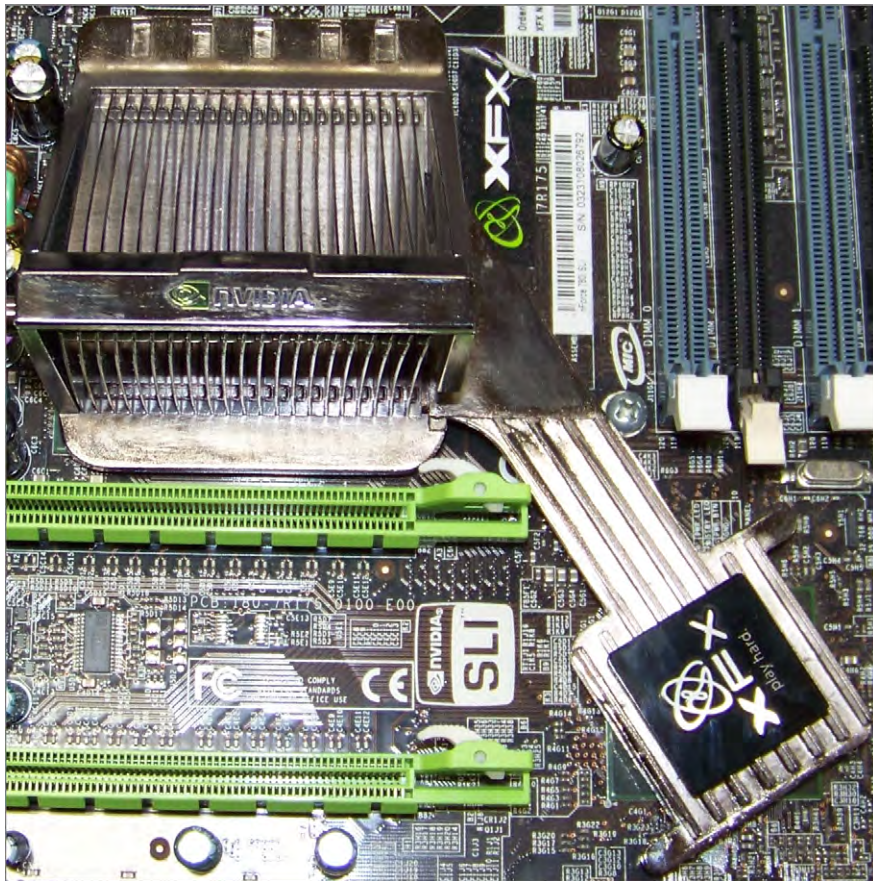
FIGURE 1.2 A modern computer chipset
