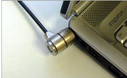
FIGURE 17.8 A cable in the security slot keeps a laptop from being taken easily.
