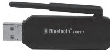
FIGURE 8.8 Bluetooth USB adapter
