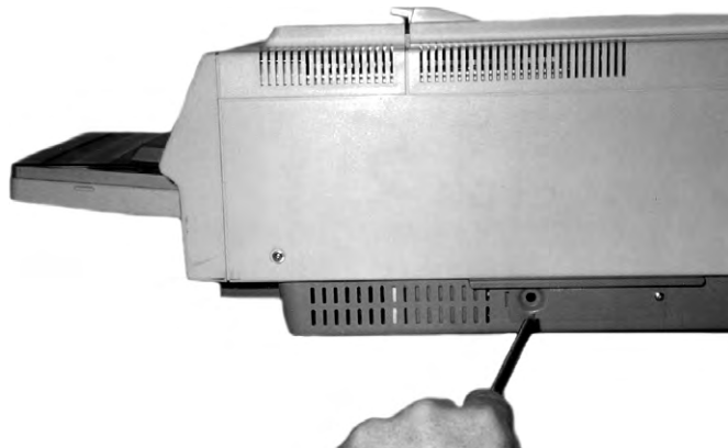
FIGURE 20.5 Print engine self-test button location. The location may vary on different printers.
