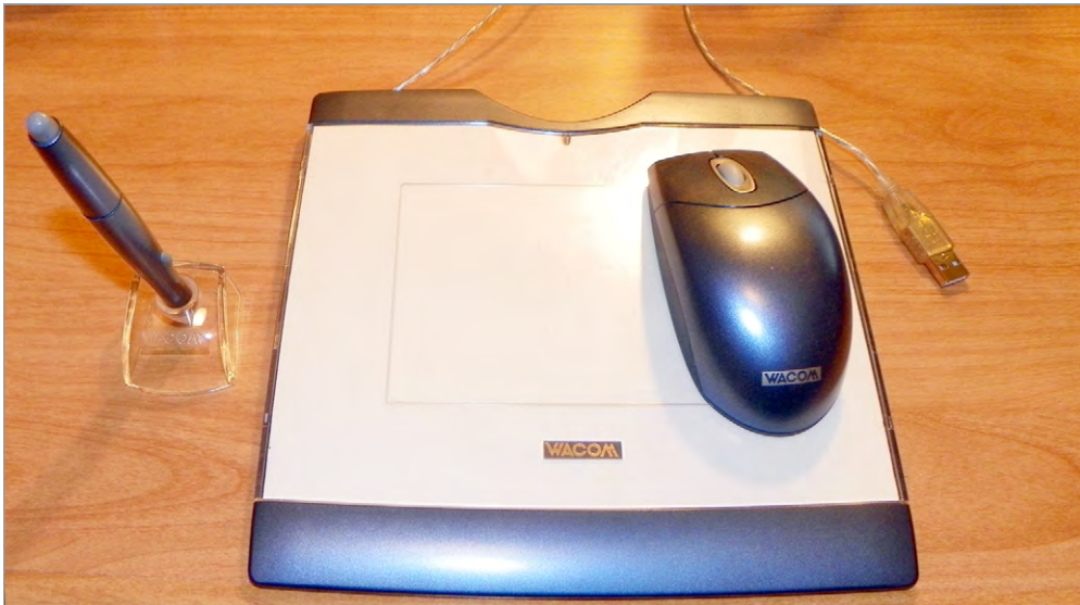
FIGURE 3.48 A digitizing tablet
