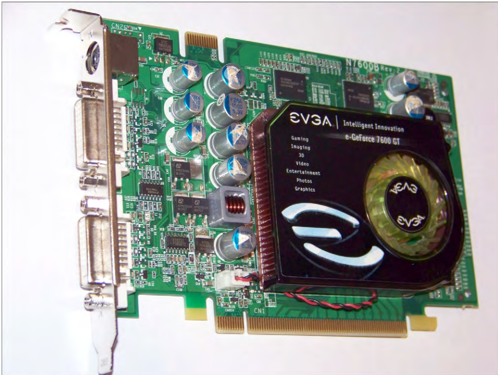
FIGURE 3.1 A video expansion card
