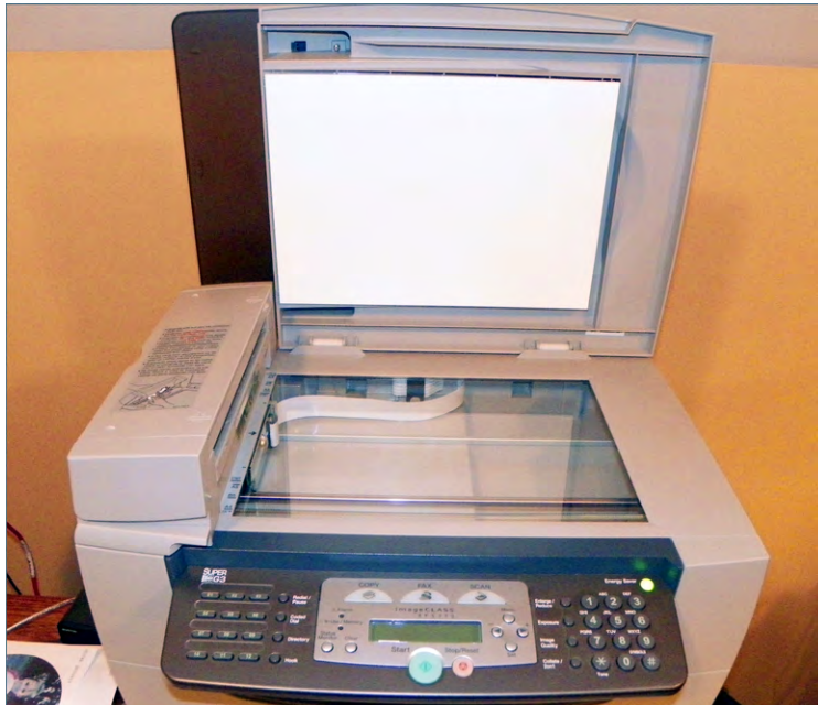
FIGURE 3.45 A flatbed scanner
