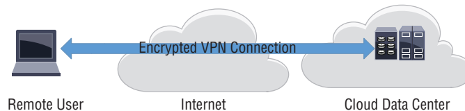
FIGURE 2.7 A VPN creates a secure tunnel over an insecure network such as the Internet.
