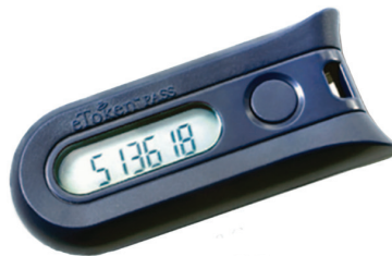
FIGURE 4.2 Hardware-based multifactor authentication token
