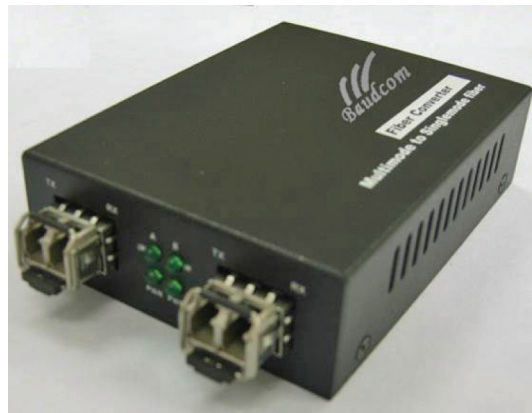
FIGURE 3.15 Single-mode to multimode fiber
