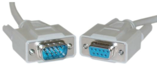
FIGURE 3.16 RS-232 cable ends
