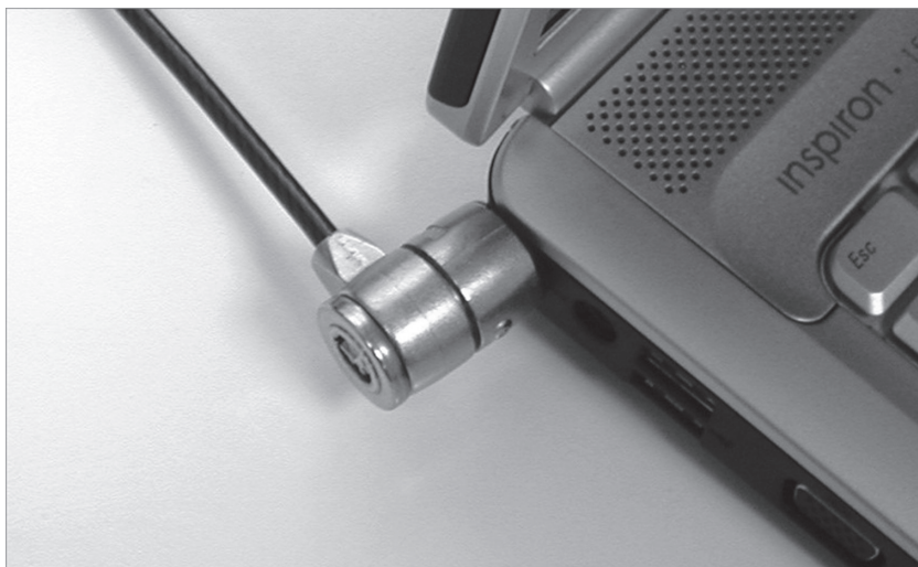
FIGURE 10.14 A cable in the security slot keeps the laptop from easily being removed.
