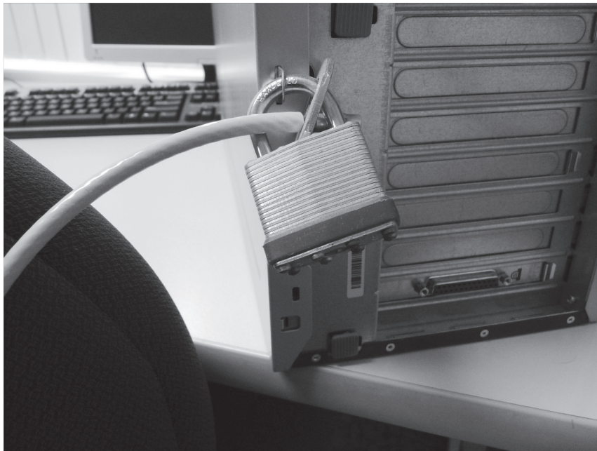
FIGURE 10.7 A cable can be used to keep a desktop machine from easily being taken.
