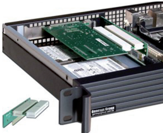
FIGURE 1.21 Riser card in rack server
