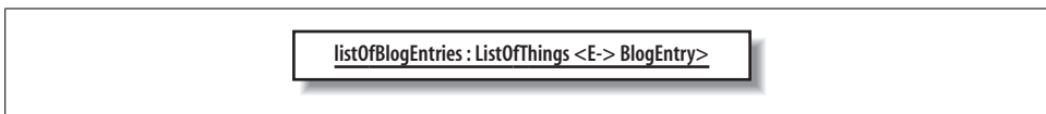
Figure 6-12. The listOfBlogEntries reuses the generic ListOfThings template, binding the E parameter to the BlogEntry class to store only objects of the BlogEntry class
