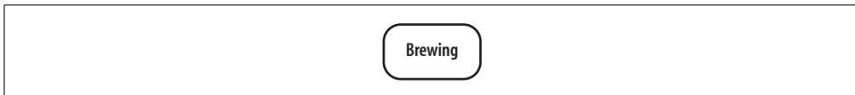
Figure 14-4. A rectangle with rounded corners and the name in the center is the most common way to draw a state
