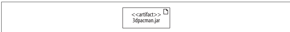
Figure 15-3. A physical software file such as a jar file is modeled with an artifact
