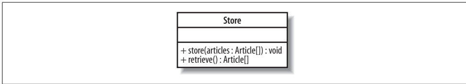
Figure 5-11. Using regular operations, the Store class needs to know how to store and retrieve a collection of articles
