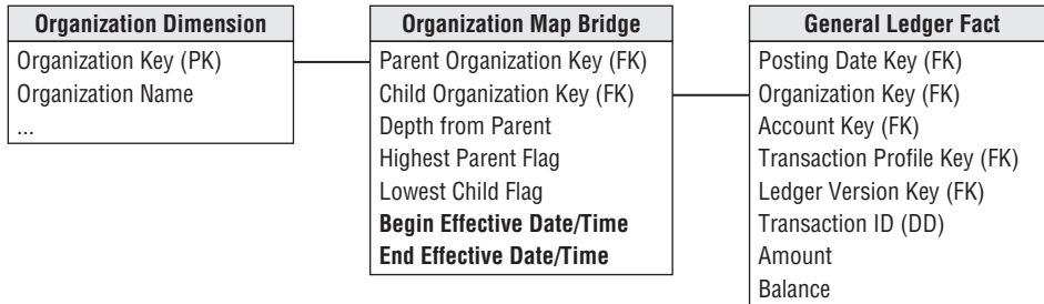
Figure 7-14: Bridge table for time varying ragged hierarchies.
