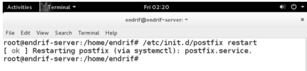
A terminal window titled 'Terminal' with the date 'Fri 02:20'. The prompt is 'endrif@endrif-server: ~'. The command executed is '/etc/init.d/postfix restart'. The output is '[ ok ] Restarting postfix (via systemctl): postfix.service.' followed by a new prompt.
