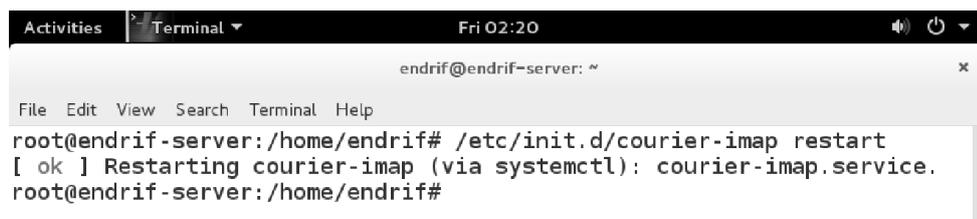
A terminal window titled 'Terminal' with the date 'Fri 02:20'. The prompt is 'endrif@endrif-server: ~'. The command executed is '/etc/init.d/courier-imap restart'. The output is '[ ok ] Restarting courier-imap (via systemctl): courier-imap.service.' followed by a new prompt.
