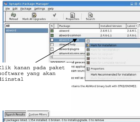
Gambar 3.13 Instal paket software
