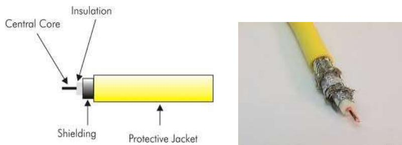
Gambar Thick Coaxial cable
